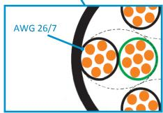
Prepared on cable with 26/7 AWG wire diameter
