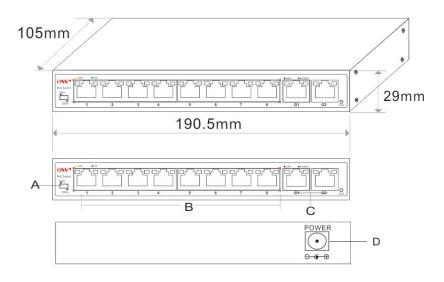
A. Multi-functional switch 100/250mB. 8\*10/100M PoE portsC. 2\*10/100/1000M uplink RJ45 portsD. Power input port DC52V
