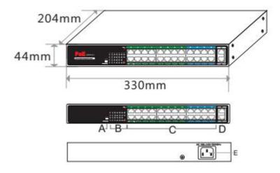
A.Multi-functional switch B.Working LED indicator C.24\*PoE port D.2\*10/100/1000M uplink RJ45 port E.Power input port AC100-240,50/60Hz
