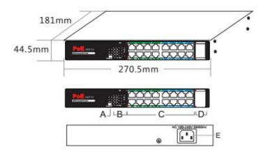
A.Multi-functional switch B.Working LED indicator
